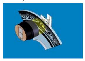
The measuring system in the single-turn module consists of a light source, a code disc pivoted in a precision ball bearing and an opto-electronic scanning device. A LED is used as a light source which shines through the code disc and onto the screen behind. The tracks on the code disk are
